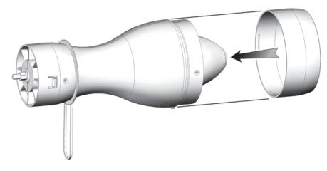
Fit the rear part of the engine body as shown. This is a tight fit, so press firmly to ensure it is in place.
