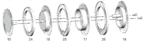
Assemble the low pressure turbine. Secure with two screws.
