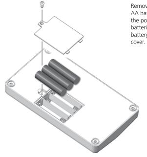
Remove the battery cover and fit 3 x AA batteries, as shown, making sure the polarity (+ and – markings) on the batteries match the markings in the battery compartment. Replace the cover
