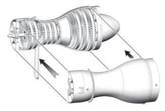
Fit the left housing (2). Hold the two halves of the engine housing together. Pull the drive belt to check that all of the compressor and turbine blades rotate smoothly.
