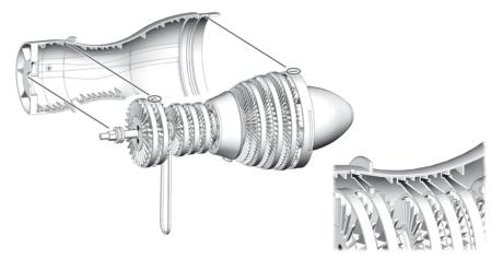
Fit the turbine assembly to the right housing (1). There are lugs in the guide vane ring (20) and the tail cone (53) – make sure these locate correctly in the corresponding slots in the housing. Also make sure that the guide vanes fit within the slots moulded into the housing – refer to the inset picture. Note that the wire from the combustion chamber exits through the slot in the bottom of the housing.
