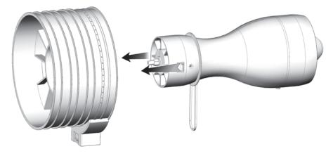
Slide the assembled engine core in to the fan housing, making sure the clips on either side engage correctly with the corresponding slots in the housing.
