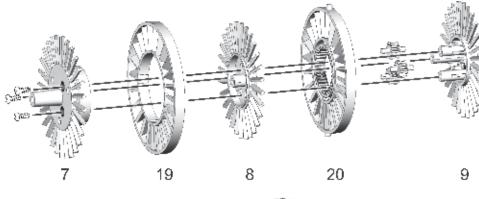
Assemble the low pressure compressor stage using the parts shown. The guide vane (19) is a loose fit over the rear of part (7) – this is intentional. Secure with three screws. We recommend that you fit the drive gears (51) to the rear of part (8) first, then fit part (20) over these (refer to inset picture).
