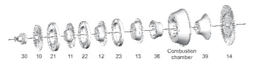
Assemble the high pressure compressor and turbine. Note how parts (38) and (39) are fitted through the middle of the combustion chamber. As in Step 1, the guide vanes (21, 22, 23) are a loose fit. Press firmly to ensure all parts are assembled correctly, but take great care to prevent damage to the fan blades.
