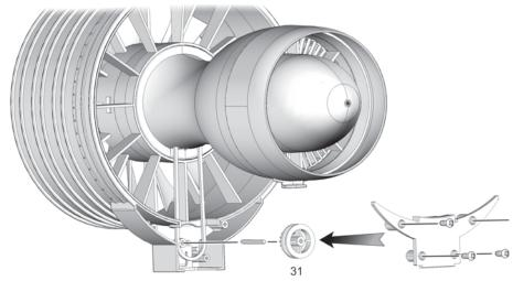
Slide the large geared pulley (31) over the short metal shaft (25 mm), and fit to the base of the fan housing. Attach the pulley cover plate (32) and secure with four screws.
