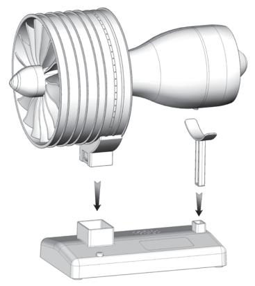
Insert the clear plastic support to the base. There are clips on one side of the support – these should face the front of the engine. Fit the engine assembly to the base/support. There is a lip on the underside of the rear of the engine which fits over the rear support. Attach this first, then carefully insert the front section into the base. Push down firmly so the drive system engages correctly you should hear it click into place.
