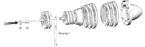
Slide the long metal shaft through the assemblies from Steps 1-4. The drive belt should be fitted to the small geared pulley (30) at this time. Finally, fit the shaft bushing A (35) and the shaft bushing B (36) to the end of the shaft.
